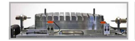
**#AUTOMOTIVE** Our dies have a thickness tolerance of less than 1/10 mm. This way, there is virtually no thickening or necking in the stamping image.
