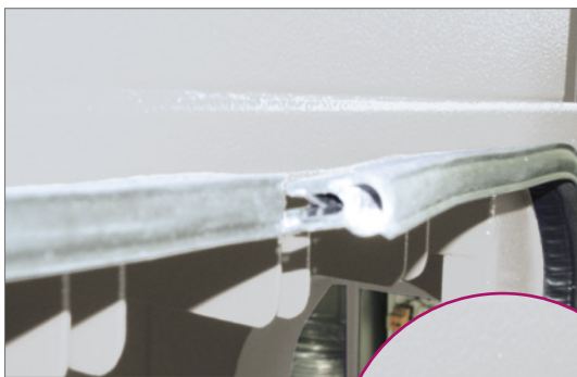
Fig.: Remove the old seal
